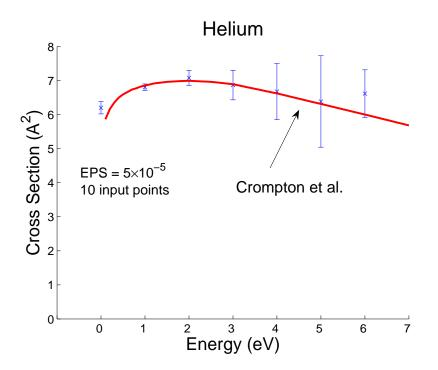
Figure 4-1: Results of GA optimization after 50 generations (data from [14]). The solid line shows the momentum-transfer cross section of Crompton *et al.*, which is in close agreement with the theoretical calculation of Nesbet [26], performed using variational methods in quantum mechanics.
