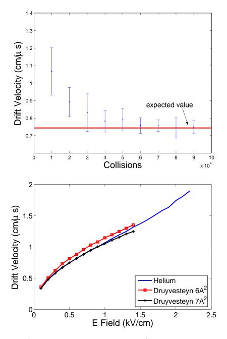
Figure 2-2: Drift velocities computed by Monte Carlo. The upper graph was computed for E = 0.5 kV/cm and  $\sigma_m = 6 \text{\AA}^2$ .
