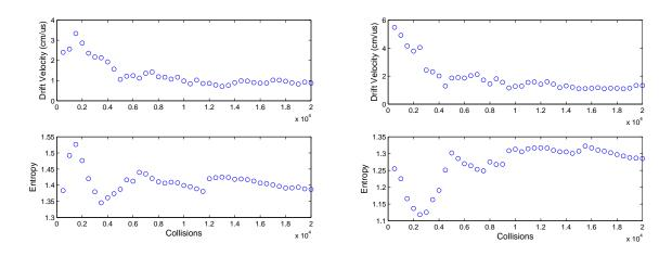
Figure 2-8: Electron-swarm thermalization, shown for simulated <sup>4</sup>He atoms. On the left, the simulated electron was subject to an applied field of E = 1.0 kV/cm; the electron on the right was driven by a field of E = 1.5 kV/cm. Note that in both cases the entropy computed using Eq. (2.11) settles to a steady value after several thousand collisions.
