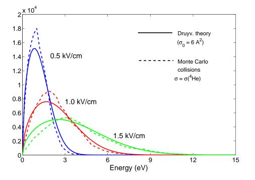
Figure 3-2: Theoretical predictions of the Druyvesteyn model compared with Monte Carlo calculations. The dashed lines indicate a histogram of collision energies, recorded during simulation runs of  $5 \times 10^5$  collisions. Note that the Druyvesteyn approximation (which is an equilibrium result obtained in the hydrodynamic regime) closely follows the Monte Carlo calculation results.
