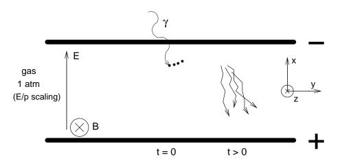
Figure 2-1: Schematic sketch of an electron swarm progressing through a drift chamber.
