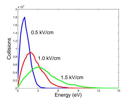
Figure 2-4: Histograms of electron collision energies at three different electric field values. Dividing by  $5 \times 10^5$  (the total number of collisions) gives the probability distribution  $h(\epsilon)$ .
