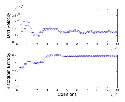
Figure 2-5: Comparison of  $v_d(t)$  and  $S_B(t)$  thermalization profiles.
