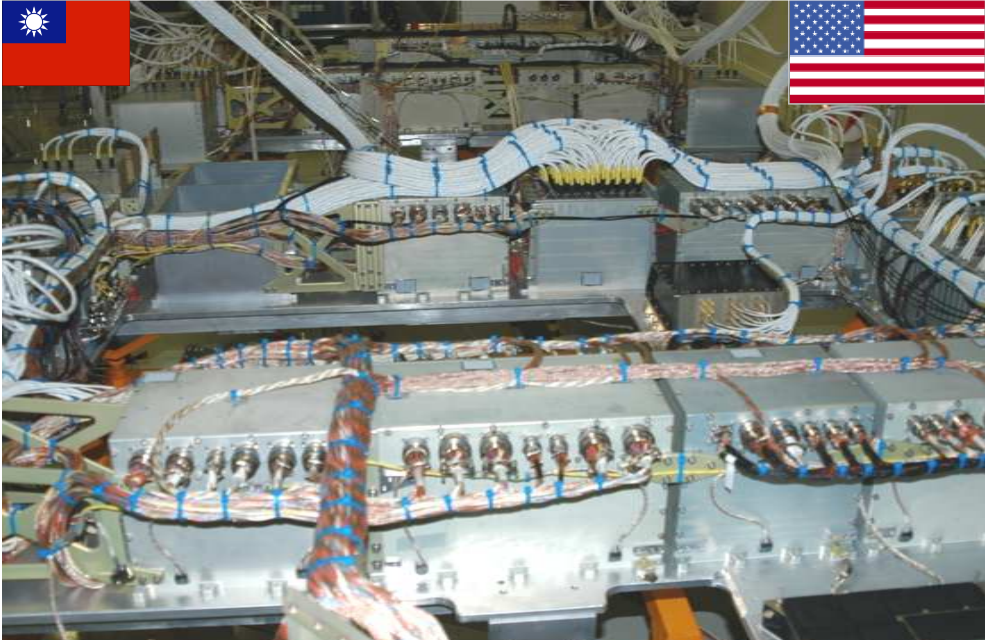
The completed flight electronics (650 microprocessors, 300,000 channels)
